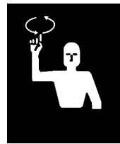
Fig. 11 - RAISE EQUIPMENT. Make circular motion with either hand at head level.
