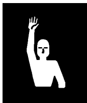
Fig. 5 - STOP. Raise hand upward to the full extent of the arm, palm to the front. Hold that position until the signal is understood.
